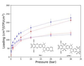
The adsorption isotherms for CO<sub>2</sub> in soPIM-1 in blue, and in PIM-1 in red. soPIM-1 is shown to have increased CO<sub>2</sub> uptake with less induced swelling compared to PIM-1, which enables adsorption processes to be operated at lower gas pressures.
